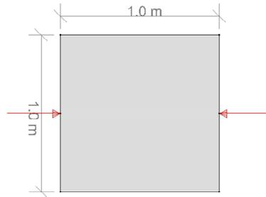
Using Diamonds (= FEM software) we calculate the stress  $\sigma_{xx,s}$  for different mesh fineness's:
