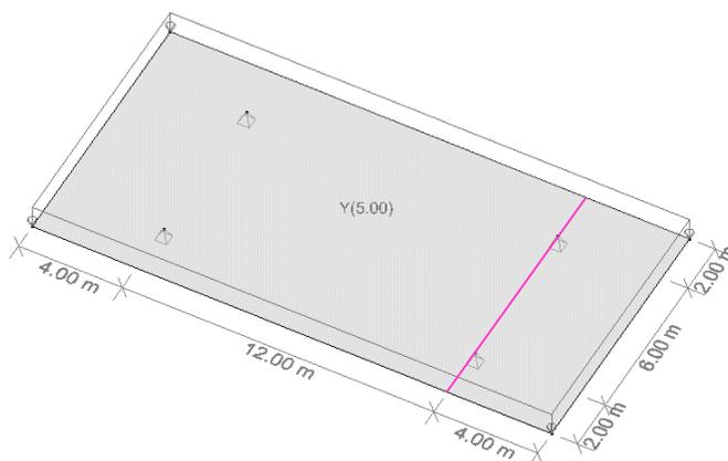
We compare the total moment along the pink cut line in Diamonds with the theoretical value 400kNm (= 5kN/m<sup>2</sup>\*4m\*10m\*4m/2) for different mesh sizes. In the process, we also compare the peak value of the moment above the supports.
